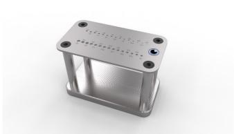
The measuring plate is made of stainless steel with a thickness of  $(2.0 \pm 0.1)$  mm. The measuring plate has a total of 30 holes with no sharp edges with a diameter of 0.6 mm up to 3.5 mm in increments of 0.1 mm. The Tolerances on hole diameter equal to  $\pm$  0.02 mm.
